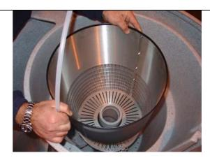
10) Align the air tube as shown, ensuring that the "Eazy" support legs are positioned equally either side of the waste drain.
