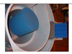
3) Remove the existing black spigot (later models having 3 retaining screws).
