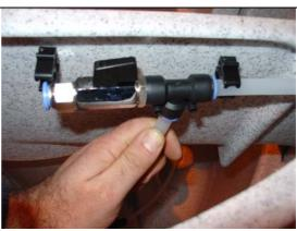
8) Connect the new backwash air tube to the "Eazy" aeration ring
