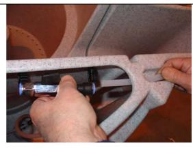
7) Connect the existing air-ring air tube to the lower connection on the "T" connector.
