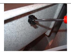
6) Remove the current 90° air-pipe elbow by pushing in the collar and pulling pipe out. Connect the incoming air tube directly to the new "T" connector.
