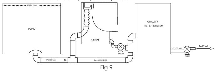
The 4" (110mm) pipe between the Cetus and the filter will allow water to pass in the direction of the higher demanding unit (it is recommended that the pump from the Cetus has a higher flowrate than the pump from the filter.
