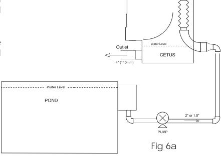
This method of installation enables the user to prefilter the pond water through the pond sieve prior to being delivered into the next stage of filtration.
