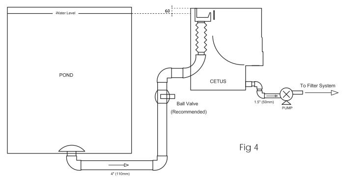
Figure 4 shows the standard way of installing a gravity fed Cetus. Figure 4a shows a gravity fed installation on a skimmer line.
