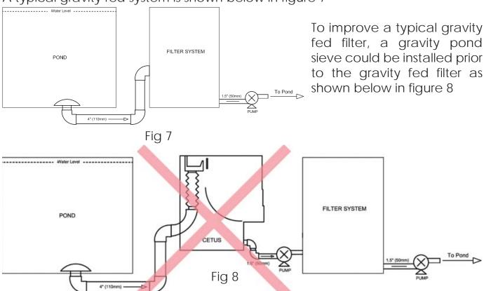
Two pumps would be used in this application. One for pumping the water from the pondsieve to the filter and the second pump for pumping water from the filter back to the pond. **The major problem** with this setup is that it is almost impossible to balance the running speeds of the two pumps. This setup can cause the gravity fed filter to overflow or have the water emptied from the filter.
