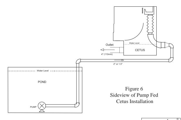
Figure 6 shows the standard way of installing a pump fed Cetus.
