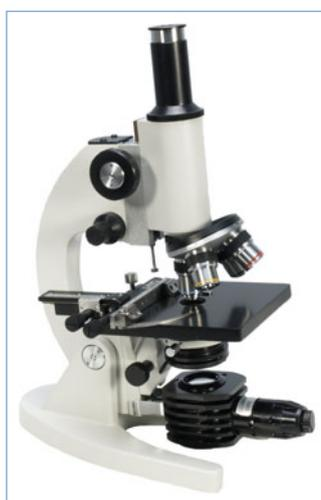
The Wedmore microscopes are a traditional shaped instrument often associated with student use and education. However the optical parts are standard and the potential specification of the Wedmore can be upgraded, to make it suitable for dark ground and phase contrast illumination.
