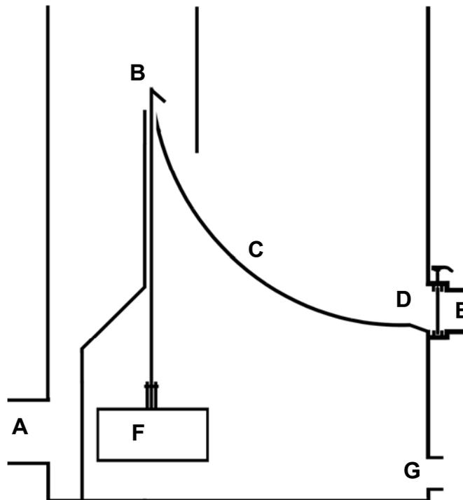
An extra advantage of this pre-filter is that the water will be provided with extra oxygen, when it goes through the slots.
