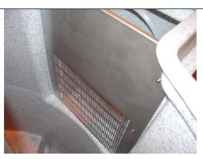
8) Refit and tighten the "Nyloc" nuts.(Ensure that the sealing washers are fitted on the outside of the tank under the heads of all screws).
