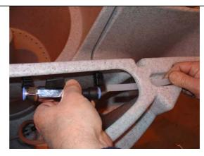
14) Connect the existing air-ring air tube to the lower connection on the "T" connector.
