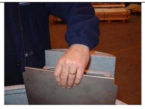
2) Remove the existing exit "D-Plate" by carefully inserting a small screwdriver through the slots in the plate and gently ease the plate upwards and out.
