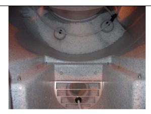
6) Fit the new weir plate over the two lower sets of screws.
