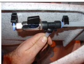
15) Connect the new back wash air tube to the other side of the air valve.
