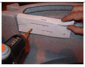
12)Fit the two air-pipe clips using the M4 screws and "Nyloc" nuts supplied.
